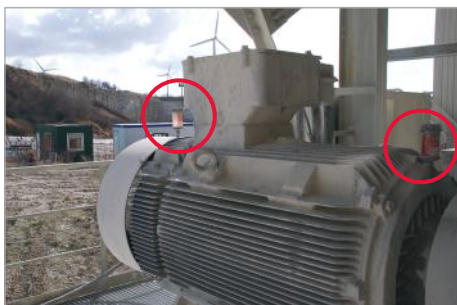
Lubrication of motor on a vibrating screen
