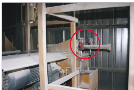
Lubrication of track roller
