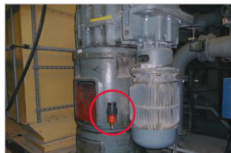
Lubrication of roller bearing on a mixer
