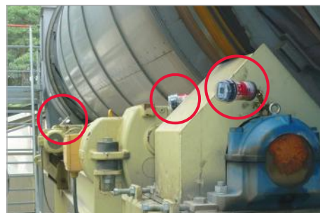
Lubrication of pillow block bearing on a rotary dryer
