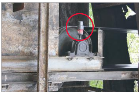
Lubrication of shaft bearing on a conveyor belt drum
