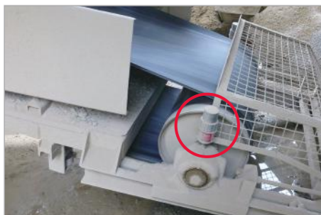
Lubrication of pillow block on a conveyor
