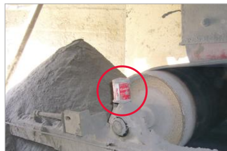
Lubrication of pillow block on a tail pulley
