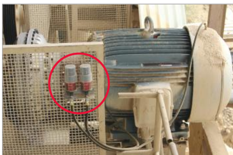
Remote lubrication of an electric motor
