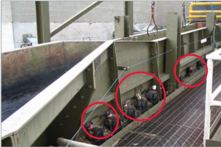
Bearing lubrication at tree sorting system
