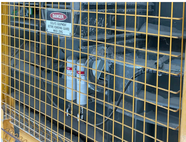
Application Travel wheels on conveyor tripper Lubricator perma STAR VARIO BLUETOOTH 250 cm 3 Installation kit K230
