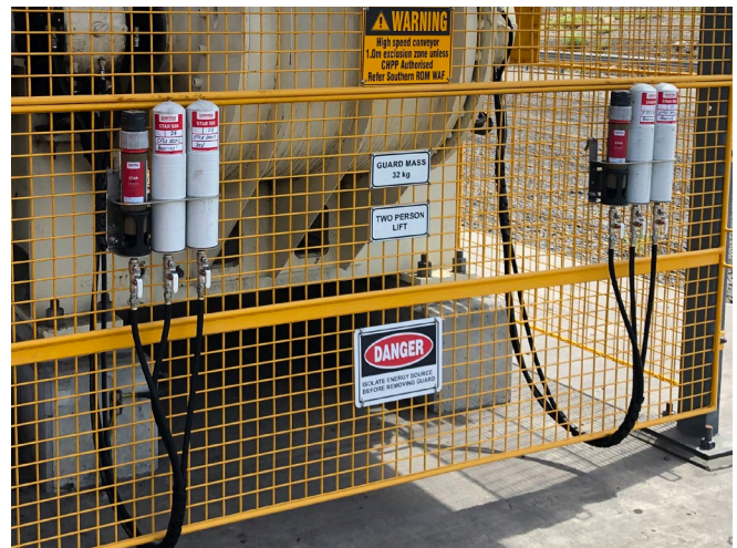
Application Conveyor pulley bearings and seals Lubricator perma STAR VARIO 500 cm 3 Installation kit 2 x K3CHCX
