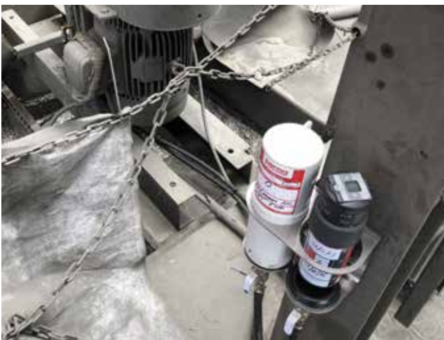
Application Sump pump Lubricator perma STAR VARIO 250 cm³ Installation kit K230C
