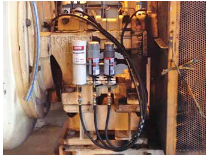
Application Labyrinth seals and gland seal Lubricator perma STAR VARIO 250 cm³ Installation kit K365C
