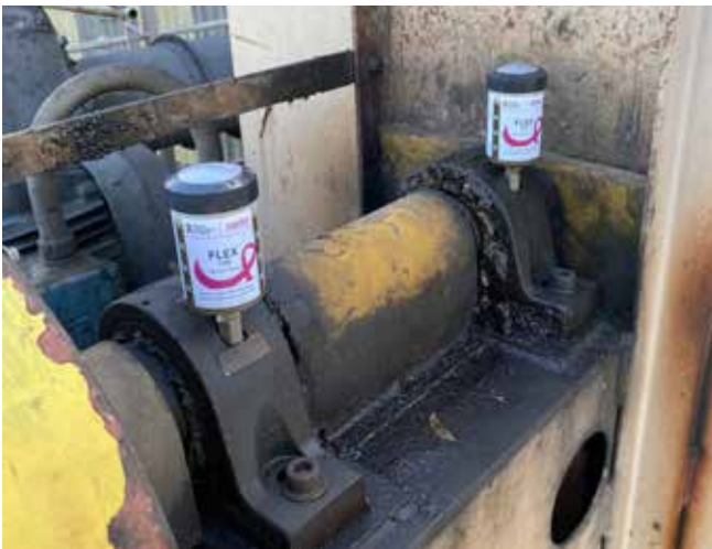
Application Fan support bearings Lubricator perma FLEX125 Installation kit Direct mount
