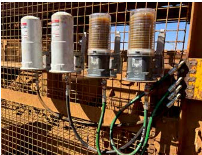
Application Conveyor pulley bearing and seal Lubricator perma ULTRA 1000 cm³ Installation kit 4 x K1UCH-1M90HD06
