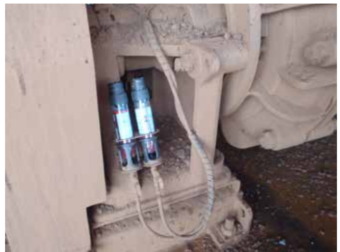
Application Labyrinth seals Lubricator perma STAR VARIO 500 cm³ Installation kit K265CX
