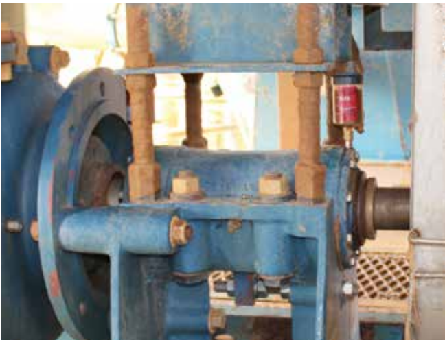
Application Labyrinth seals and mechanical seal Lubricator perma FLEX125 Installation kit Direct mount
