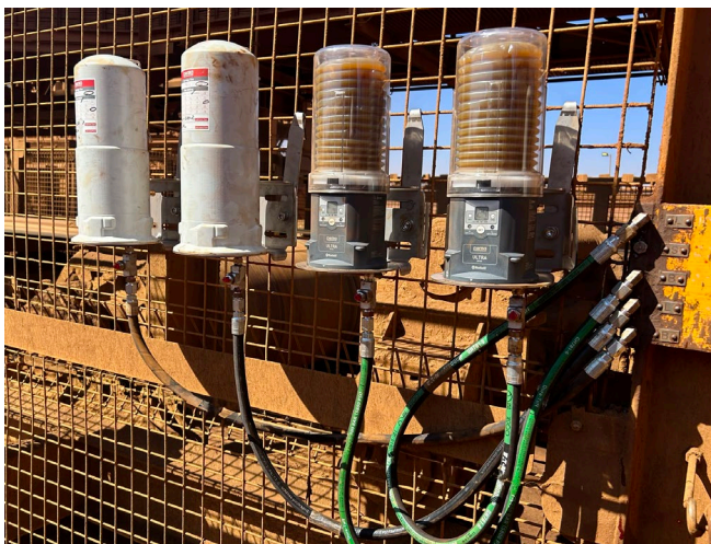
Application Conveyor pulley bearing and seal Lubricator perma ULTRA 1000 cm 3 Installation kit 4 x K1UCH-1M90HD06
