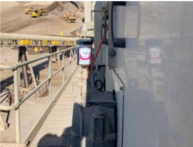
**Application** Conveyor pulley bearing and seal
