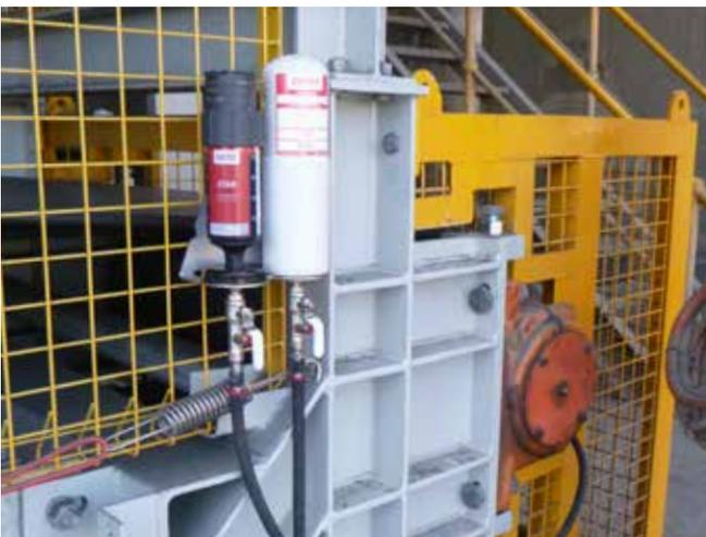
**Application** Conveyor pulley bearing and seal
