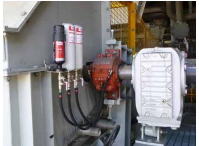
**Application** Conveyor pulley bearing and seal
