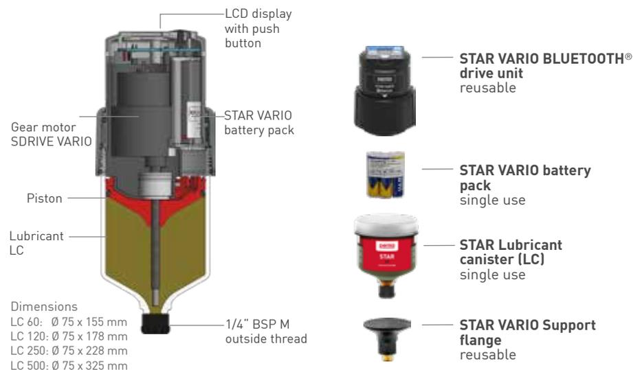
\* Total resistance to grease flow must be less than the pressure delivery capability of the lubricator
