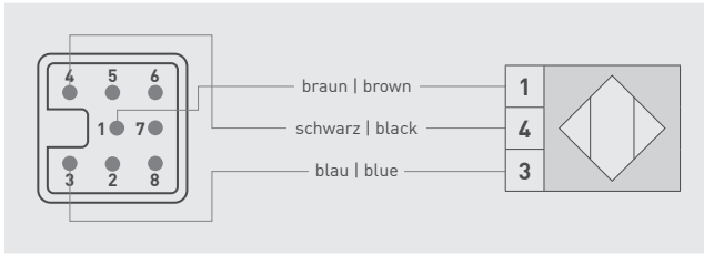
Fig. 10-5 Circuit diagram for connecting the perma ECOSY Control sensor
