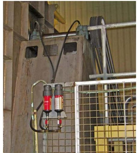
**Strategy 2** – Remote mount lubrication systems used for conveyor pulley bearings which are located behind cages to avoid unnecessary manual handling of cages.
