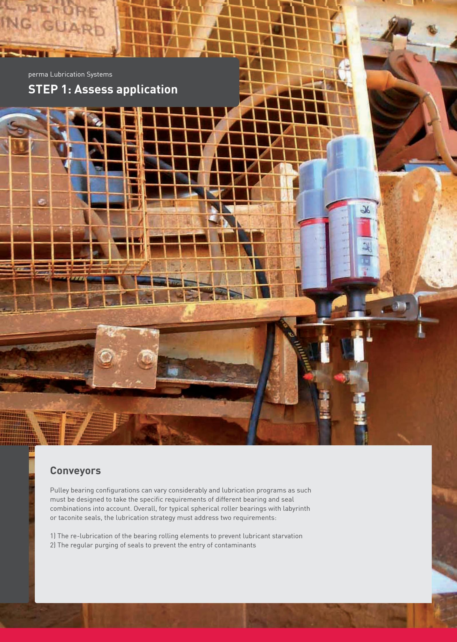
A photograph showing a conveyor system with a yellow safety cage. A blue perma Lubrication Systems dispenser is mounted on the side of the conveyor. The dispenser has two blue canisters and a red label with the number '26'. The background shows the metal structure of the conveyor and a sign that says 'BEFORE OPENING GUARD'.
