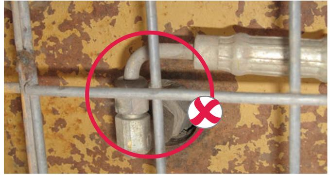
perma STAR VARIO lubrication systems have a G1/4 male thread at the grease outlet. Where reducers, elbows or extensions are required to simplify installation it is important to adhere to the following guidelines:
