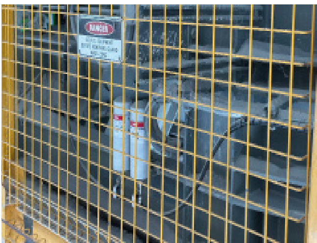
Application Travel wheels on conveyor tripper Lubricator perma STAR VARIO BLUETOOTH 250 cm³ Installation kit K230
