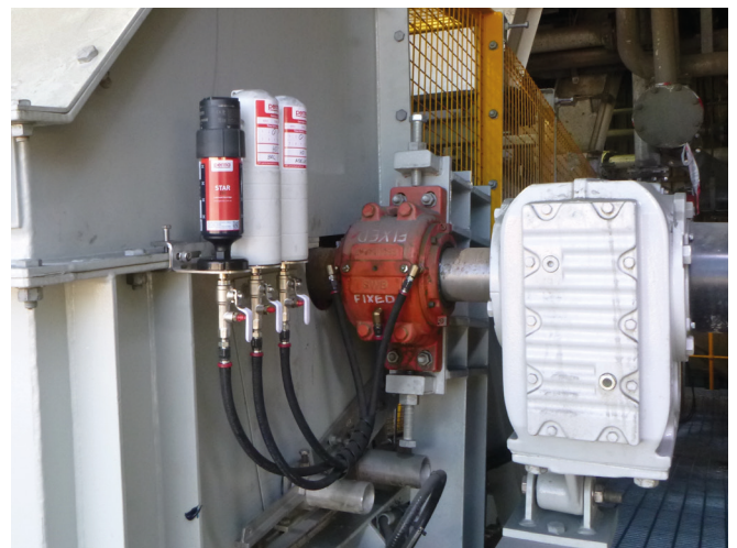
Application Conveyor pulley bearing and seal Lubricator perma STAR VARIO 250 cm³ Installation kit K330
