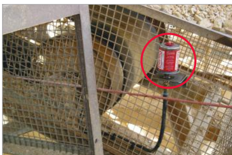
Lubrication of pillow block on a conveyor
