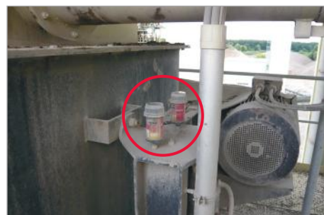
Lubrication of pillow block on a conveyor
