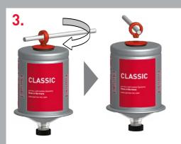
Using a tool such as the shaft of a screwdriver continue to rotate the activator until the eyelet shears off. **DO NOT** snap the eyelet off by pushing to the side. Use a **ROTATING ACTION ONLY**.
