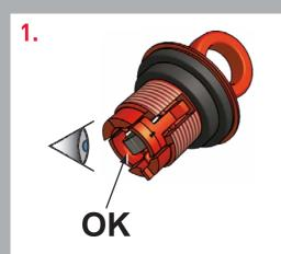
Check that the activator is in good condition and that the activation pellet is in place.
