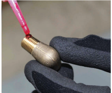
Apply thread sealant to fittings
