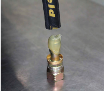
Apply grease to hose end tails before attempting to push on hose
