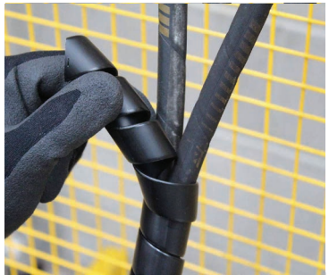
Apply spiral wrap to hoses to protect them from rubbing and to reduce catch hazards
