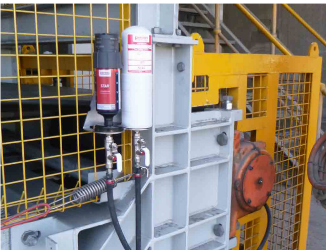
Application Conveyor pulley bearing and seal Lubricator perma STAR VARIO 250cm 3 Installation kit K2CH
