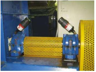
Application Fan support bearings Lubricator perma STAR VARIO 120cm<sup>3</sup> Installation kit Direct mount
