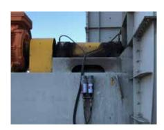
Strategy 2 - Automatically lubricate equipment which would otherwise require working at heights or confined space permits.
