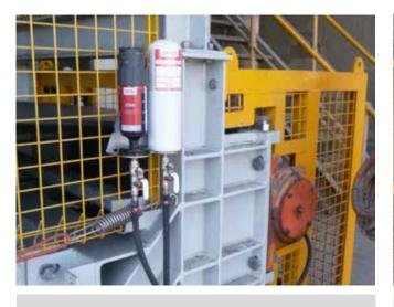
Application Conveyor pulley bearing and seal Lubricator perma STAR VARIO 250cm³
