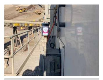
Application Conveyor pulley bearing and seal
