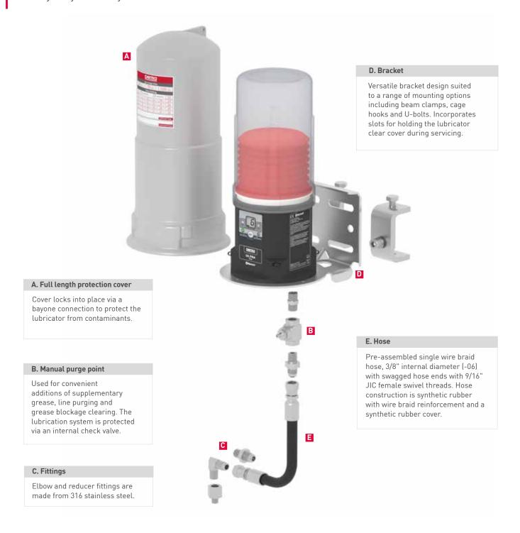
The perma ULTRA must be remote mounted, providing the opportunity to install the system at a safe and easy to access location. Installation kits include pre-assembled hose and a range of easy to use attachment options. Installation kit part numbers indicate the length of the pre-assembled hose in meters. Care should be taken to order kits with suitable hose lengths because in-field adjustment is not practical.
