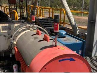
**Application** Electric motor Lubricator perma STAR VARIO 250cm³ Installation kit Direct mount
