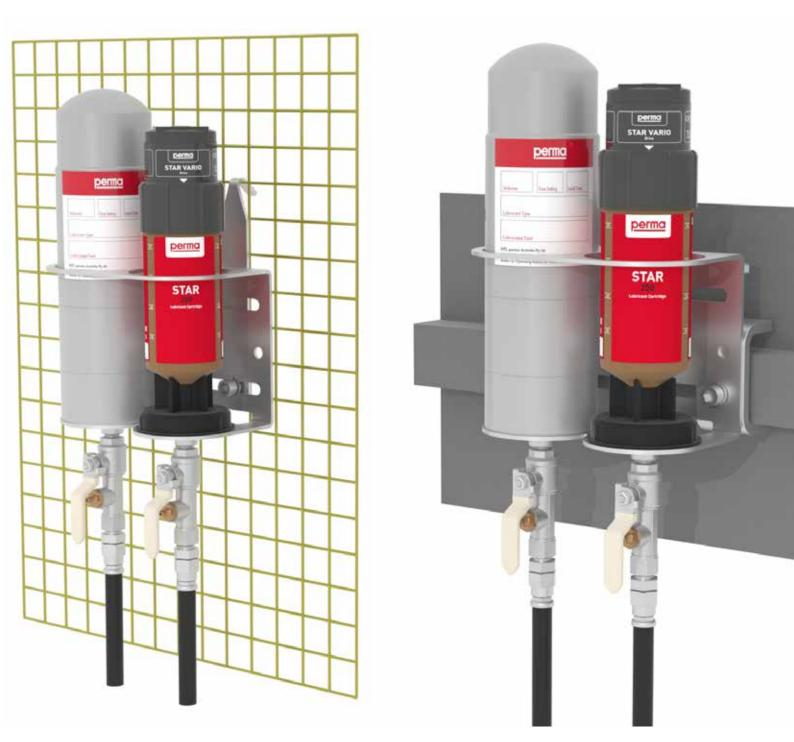
Heavy Duty installation kits have been specifically designed for use in operational areas which are subject to regular wash down and water impact, such as the conditions found in coal handling preparation plants. The installation kits are highly versatile and can be adapted for attachment to beam sections and square mesh safety cages. The bracket systems included in Heavy Duty installation kits are fabricated in Australia from stainless steel.
