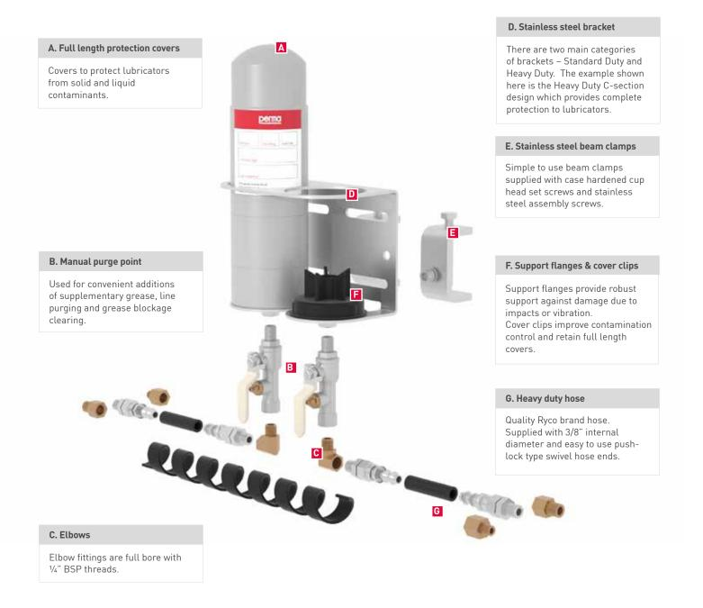
Remote installation kits are designed to be installed with maximum efficiency. Kit brackets and covers have been designed to provide suitable protection to the lubricator against accidental damage and contamination build-up. Grease line type and fittings have been carefully selected to minimise resistance to grease flow.
